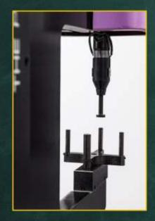
Safety sensors mounted on ram head ensures fast and safe production cycle.
