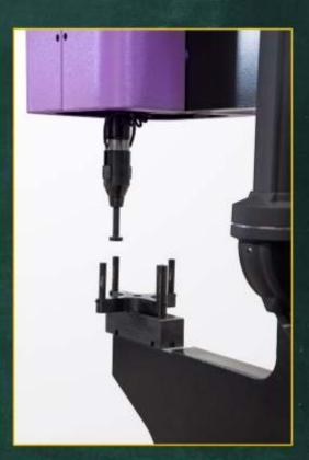
M-station turret-carousel to hold fasteners. Also available with swing arm cup table for easy pick up of parts.
