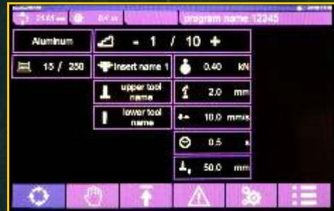
Operator friendly and powerfull TC 12 control. Easy to use and also allows modifications according customer demands. With programmable insertion speed for soft and fragile parts.
