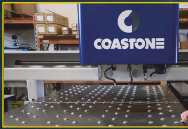
MultiTapper MT1212 chipping operation against rigid anvil.
