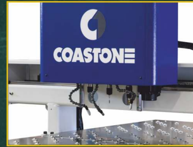
MultiTapper MT1212 for tapping and counter sinking.
