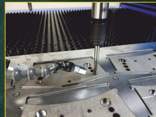
TapOne 1212. Silent tapping on brush table.
