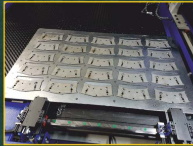
TapOne 1212. Positioning with clamps.
